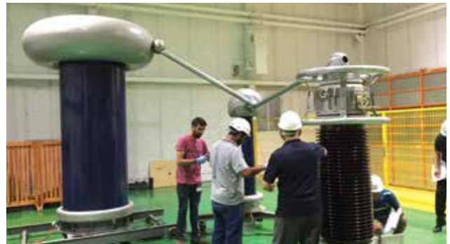
CT & IVT FAT at EMEK Electrical Industry Inc, Turkey
