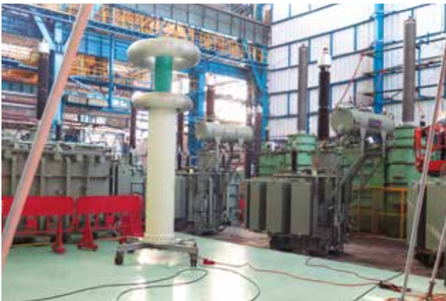
10 MVar 275kV Shunt Reactor FAT at CG India
